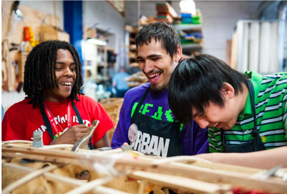
Youth instructor connects with new apprentices as they complete the box lashings that hold together the framework of a 17-½' skin-on-frame canoe.
